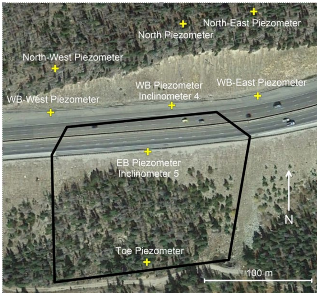
Figure C.1. Piezometer locations with approximate slide extents shown in black (from Hinds, 2018).
